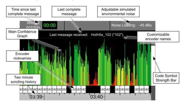
Our proprietary algorithms constantly analyze the input signal, looking for valid code symbols that the system combines to build meaningful station identifications. The input can be any real-world source: your off-air signal (or a competitor's), a test file from a production studio, an Internet stream, or even a live mic listening to a sample radio or a public space<sup>7</sup>. If there are symbols hidden in the audio, TVC-15 will report their details.
